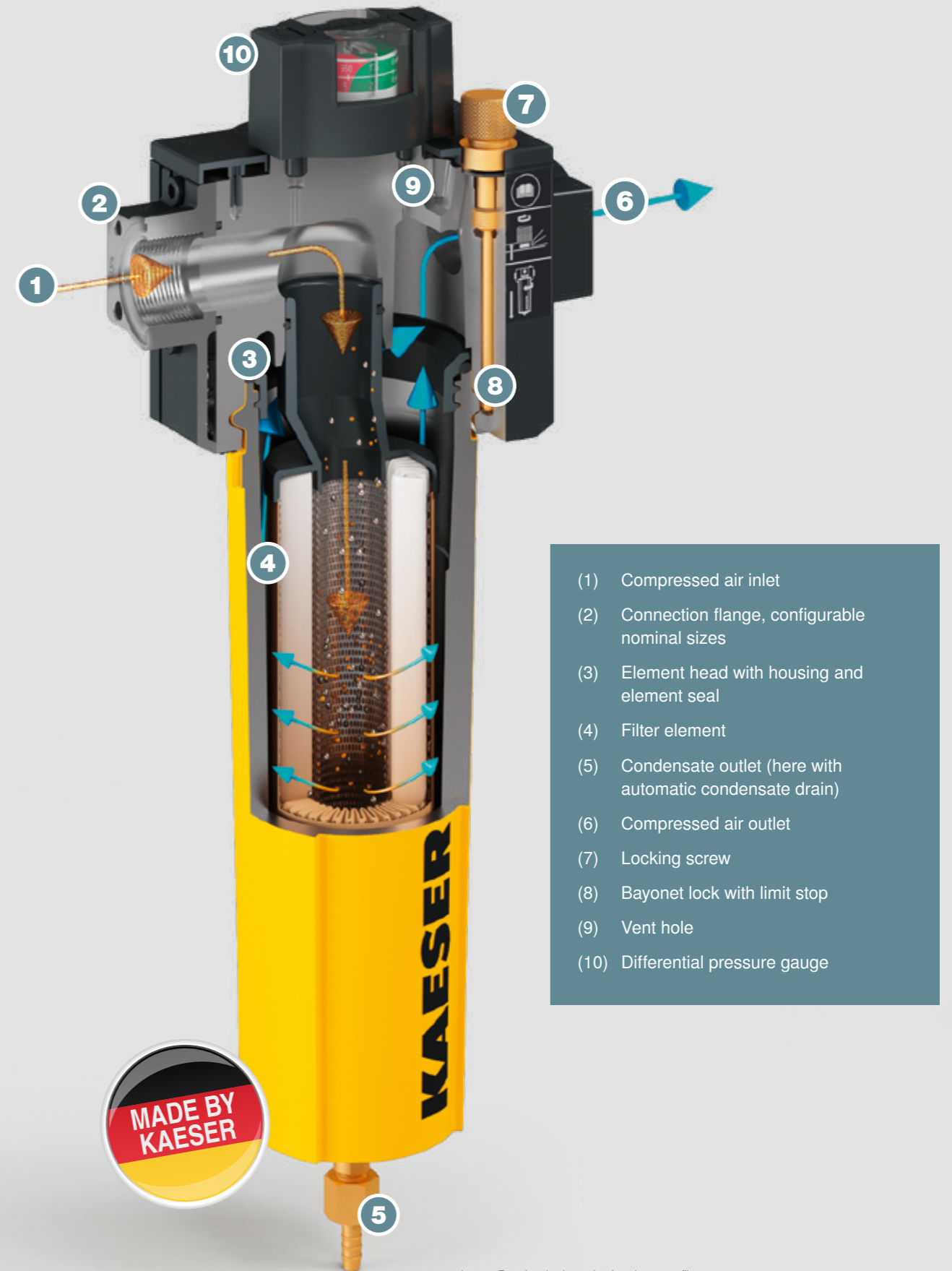
Image: Functional schematic of coalescence filter
