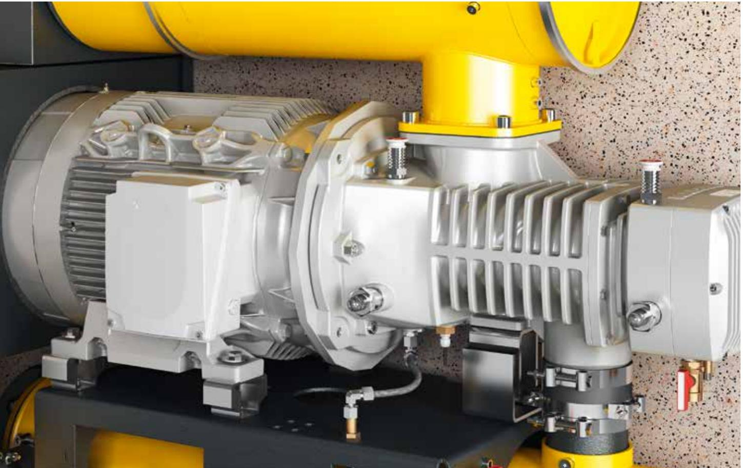
In CBS and DBS series rotary screw blowers, power is transferred from the motor to the blower airend via an integrated gear transmission. This was found to be the most effective transmission solution for the speeds in this power and size class with regards to efficiency, dependability and durability. With HBS series blowers, power is transferred directly without loss via a coupling. These concepts were the result of extensive research at KAESER's Research and Development Centres.
