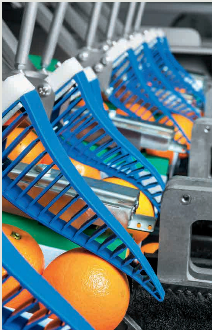
Gentle transport: the patented system from Giró with flexible gripper fingers DHAS from Festo.
