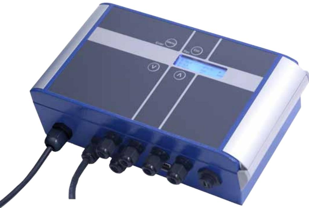
The VPFlowTerminal is a plug & play wall mount display with built-in power supply and 2 million point data logger. The VPFlowTerminal has five sensor inputs: one input for a VPFlowScope in-line or VPFlowScope insertion meter, and four generic analog inputs. It can record up to 8 channels. This makes the collection and analysis of your compressed air data easier and quicker!
