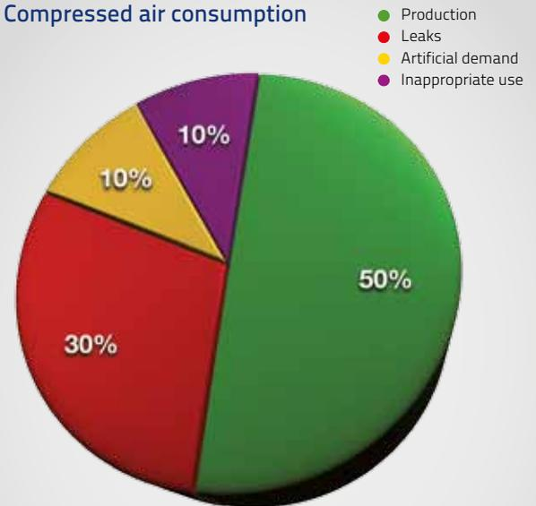
Fact: Only 50% of the generated compressed air is used usefully. The other 50% is being spilled. A management system will help you to reduce this waste of energy and money, and helps you to maintain your consumption as low as possible.
